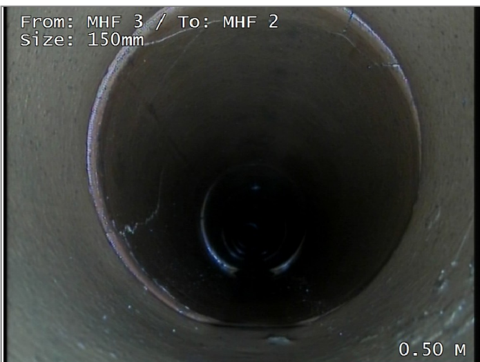
Cracks multiple from 12 to 12 o'clock
